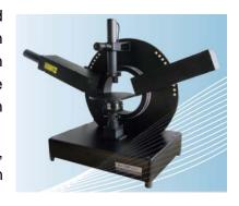
thickness and optical constants at the He-Ne laser wavelength 632.8 nm with an extraordinary precision and accuracy. The REMPro can be utilized to characterize single films, multiple layer stacks (1~3 layer) and bulk materials (substrates).
